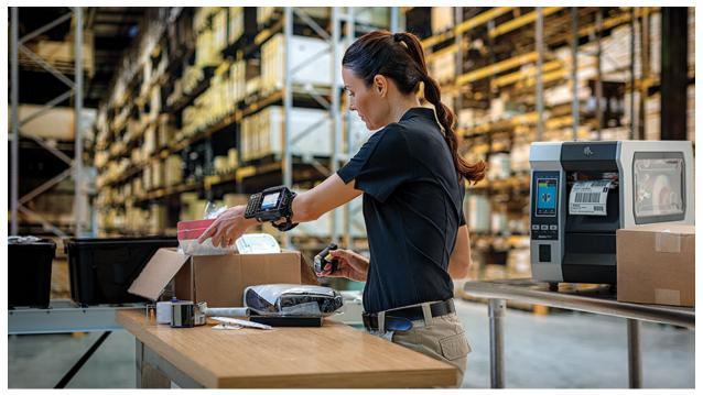
Traditional voice-directed picking can be combined with a wearable display that allows the picker to confirm a pick.
