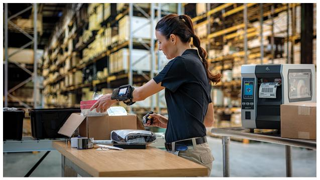
Traditional voice-directed picking can be combined with a wearable display that allows the picker to confirm a pick.
